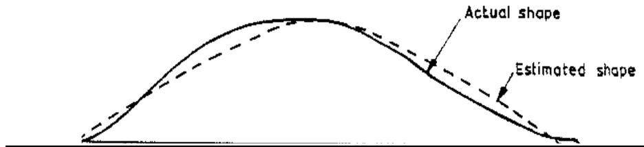
Fig. 2 Comparison between the actual waterplane shape of a ferry in the inclining condition and the shape given by Munro-Smith's approximate formula.
