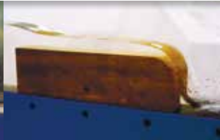
Broad crested weir - (supplied)
