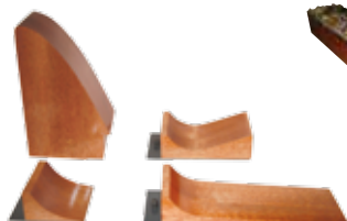
C4-64 Free overflow spillway section complete with ski jump, sloping apron and blended reverse curvature attachments
