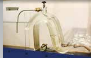
C4-65 Syphon spillway
