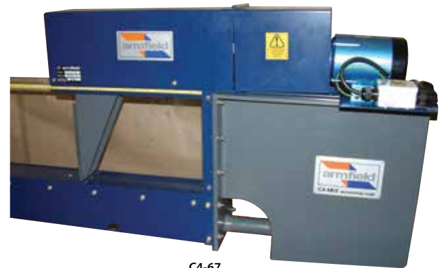
C4-67 Wave generator and *wave absorbing beach
