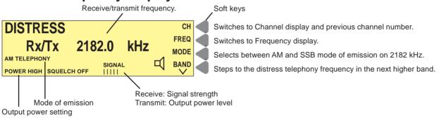
The frequencies for distress and safety telephony traffic are 2182 kHz, 4125 kHz, 6215 kHz, 8291 kHz, 12290 kHz, 16420 kHz
