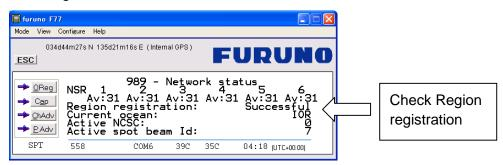
Check the Region registration field. If all communications are not established, "Failed" may be indicated. If communication fails in spite of "Successful" is indicated, contact FURUNO.
