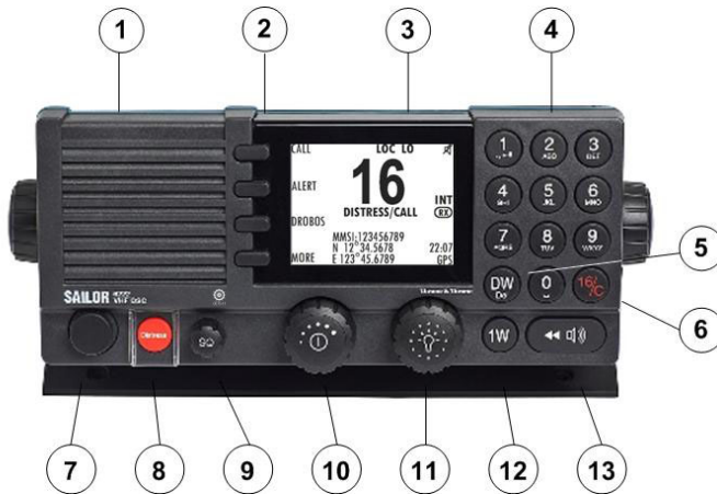
Figure 1: Controls on the front plate
