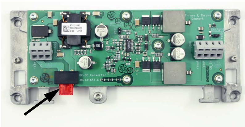
Figure 5: Replacing the fuse in the Power Converter
