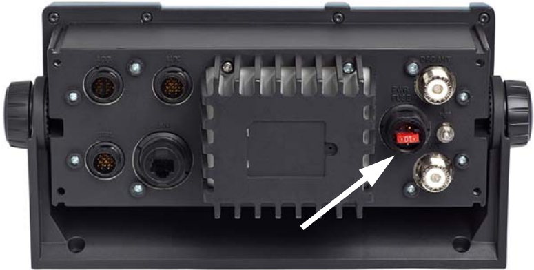
Figure 4: Replacing the fuse in the power connector
