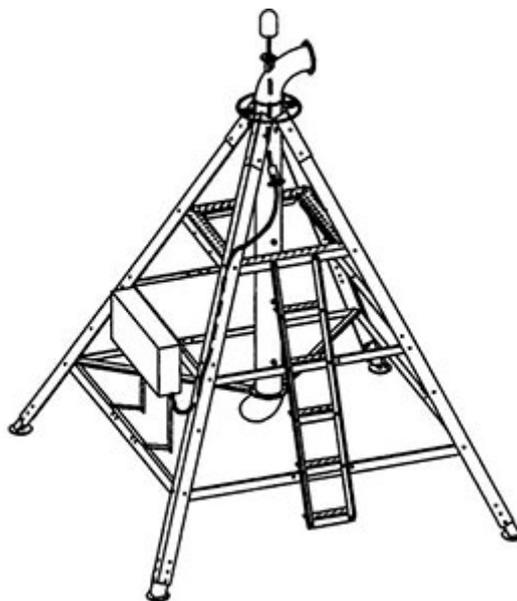
Fig 21. Torre control pivote central
