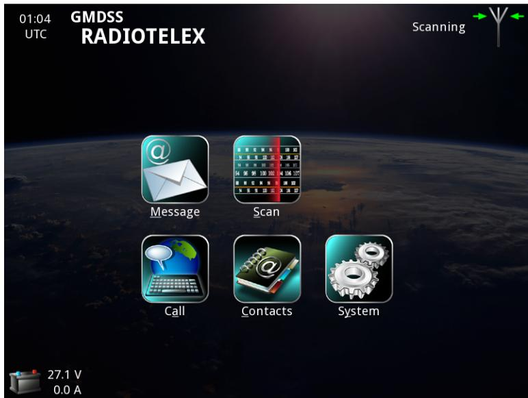
The Radiotelex application starts up automatically when the Message Terminal is powered. Note that the Message Terminal must always be powered in a GMDSS system.
