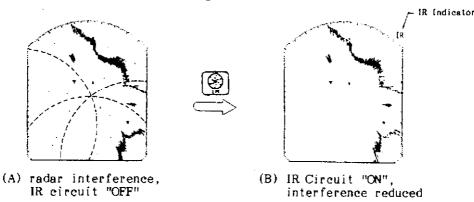
Fig.30 Radar Interference
