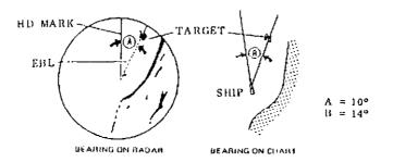
Fig.13 Relative Bearing Alignment (When the relative bearing of a target measured on the radar screen (A) does not agree with that measured on the navigation chart (B).)
