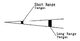
Fig.39 Beamwidth vs. Target Appearance
