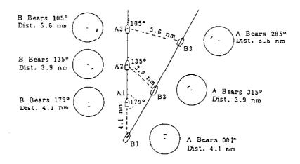
Fig.48 Relative Motion vs. True Motion
