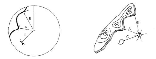
Fig.45 Position Fixing Using Radar Ranges
