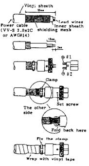
Fig.11 Power Connector Assy.
