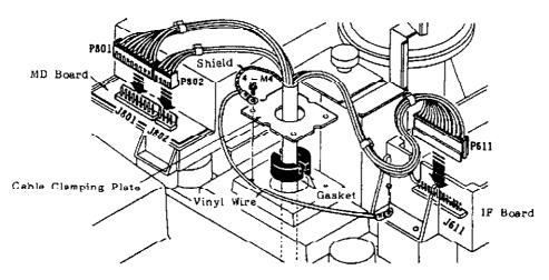
Fig.7 Cable Connection and Grounding
