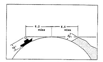
Fig.38 Radar Horizon
